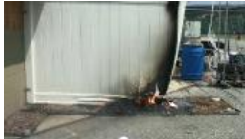
Distance to shed = 0 ft (0 m) Wind speed = 20 mph (10 m/s )
