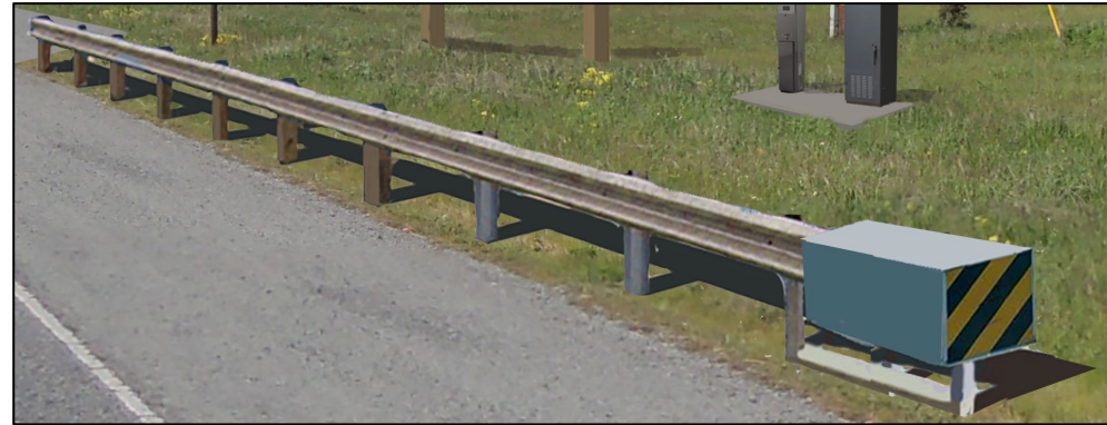
Midwest Guardrail System
